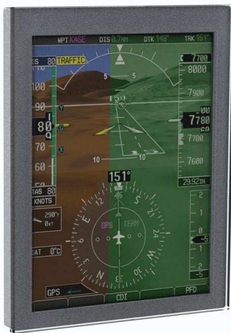
The ruggedization of the LCD include the following enhancements. Indium Tin Oxide (ITO) coated Glass with Alumnium Busbars which will act as the heater. Woven Wire Mesh placed above provides the the EMI shielding. Anti Glare Glass with Broad/Band Anti-Reflective(BBAR) Coating reduces the glare.All the above items are glued to the LCD using an optically clear adhesive (OCA)
